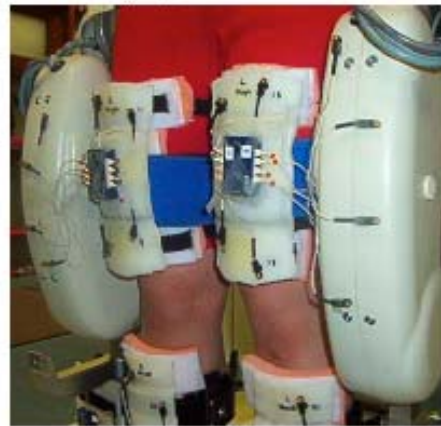
Figure 2. Active tracking markers placed on the Lokomat and custom marker clusters.
